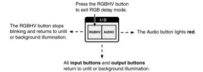
Figure 3-41 — Deselect RGB Delay mode
